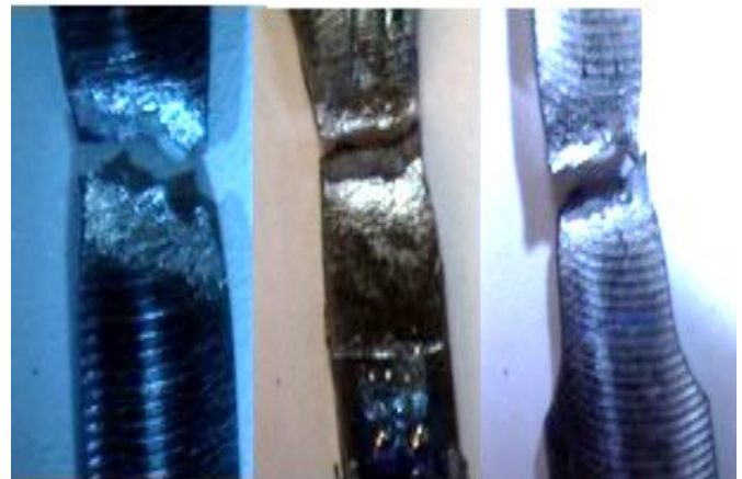
Figure 8. Type-V Specimen Necking (ductile behavior)
