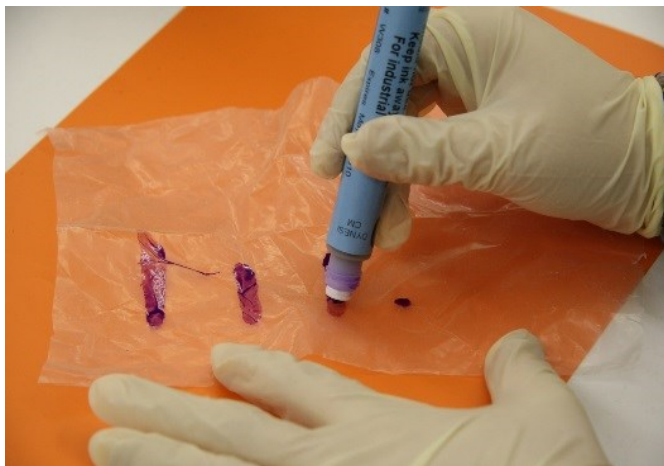
Figure 3. Illustration of the Use of an Accudyne Pen
