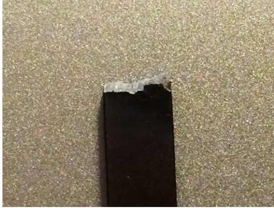
Figure 9. Type-T Specimen with a Sharp Edge (brittle behavior)
